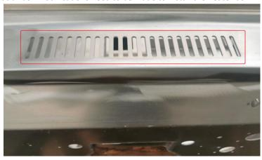
Heater box gasket must be removed (highlighted in red below)
