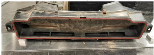
This creates a gap approximately 1/4" tall, allowing passenger cabin air to enter the heater box before re-circulating to the outlets.
