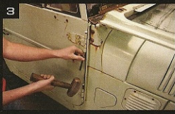
Pic 3: Now it's time to remove the OEM steel doors. Using a punch, tap the hinge pins out of the hinges. You need to fold the windshield down (or at least forward a bit) to be able to get the pins up and out of the top hinge.
