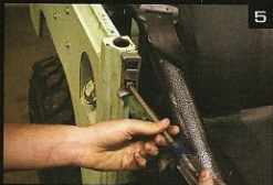
4 Pic 4: Reach inside the kick panel access and remove the bolt and pins holding the doorstop in. With the hinges unpinning and the doorstop disconnected, the OE steel doors lift right off.
