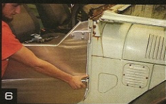
6 Pic 6: The Aqualu door is now set into place on the OE hinge halves and the OE pins are tapped into place. We could then shut the door, align the hinges up straight and tighten them securely. We also took a couple minutes to apply weather stripping tape to the inside of the half doors. That's it; total install time, about 20 minutes per door. ✓
