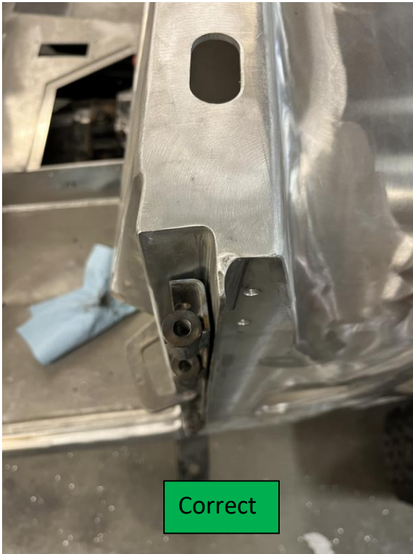
Figure 4: Correct Mounting Orientation
