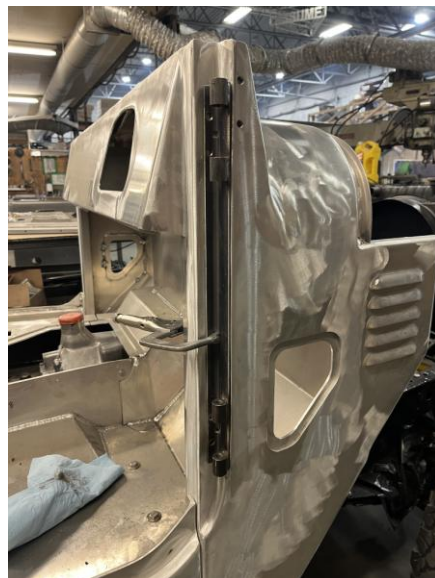
Figure 3: Aqualu Front Door Hinge Mounting
