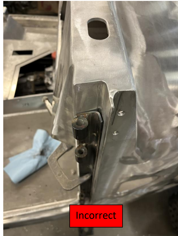
Figure 5: Incorrect Mounting Orientation
